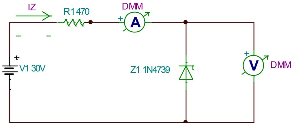
**Fig 2.1 (a) Zener test circuit**
