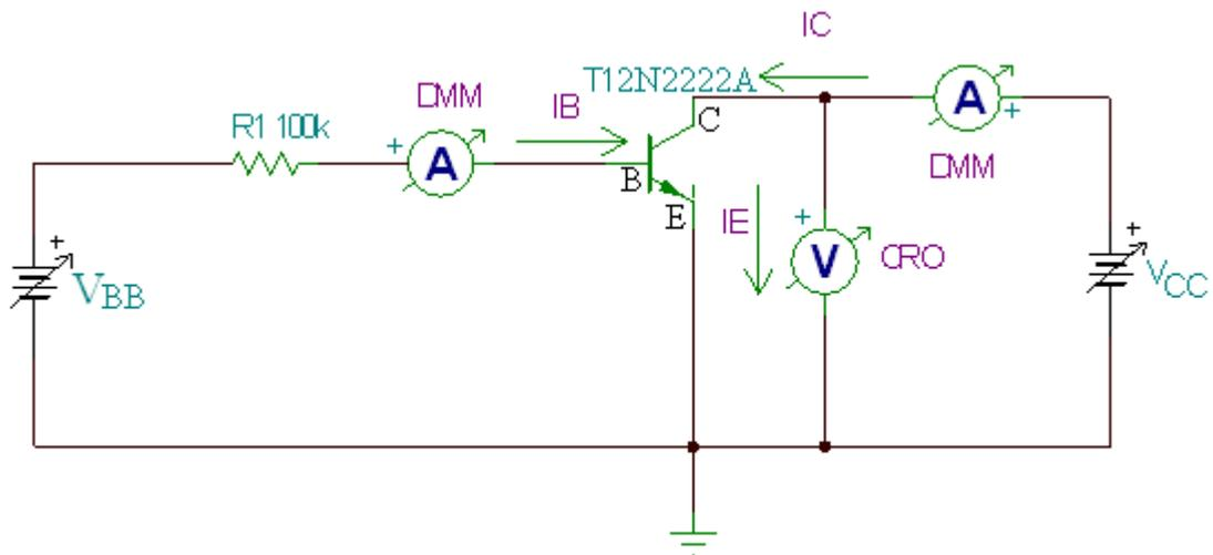
**Fig 6.2 Circuit for Common Emitter Output Characteristics**
