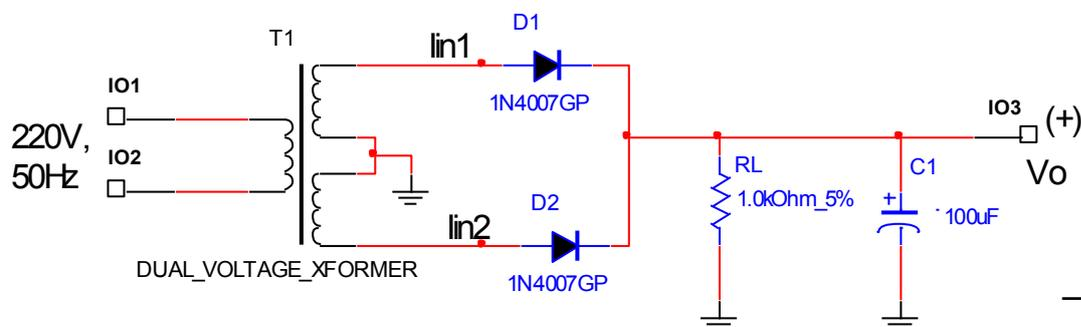
**Fig4.1 Full wave rectifier with a Capacitor Filter**
