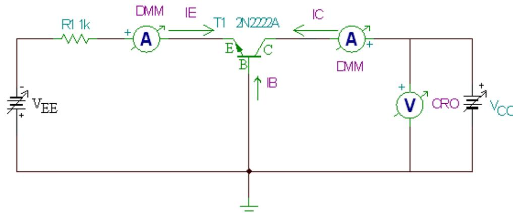
**Fig 5.2 Circuit for Common Base Output Characteristics**
