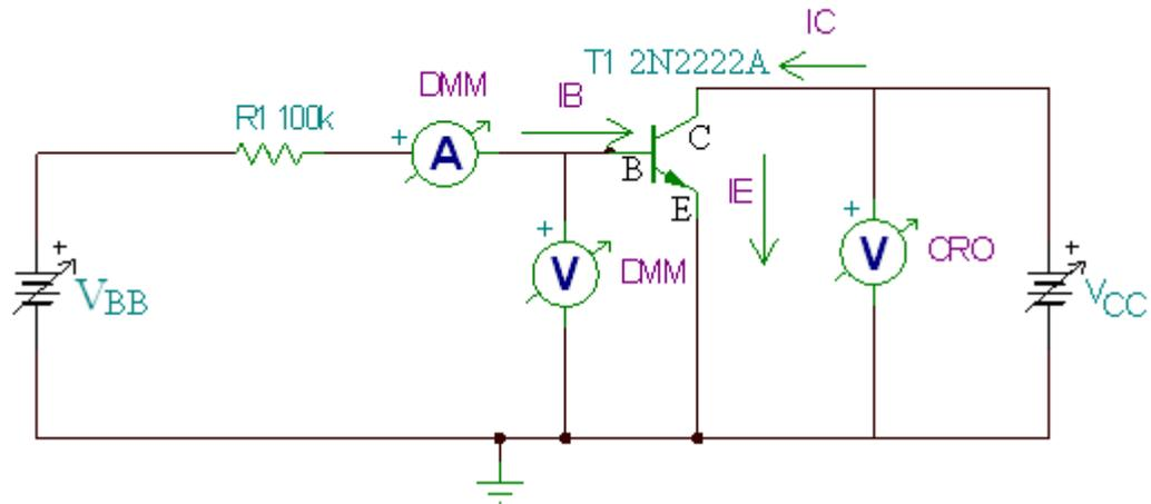
**Fig 6.1 Circuit for Common Emitter Input Characteristics**
