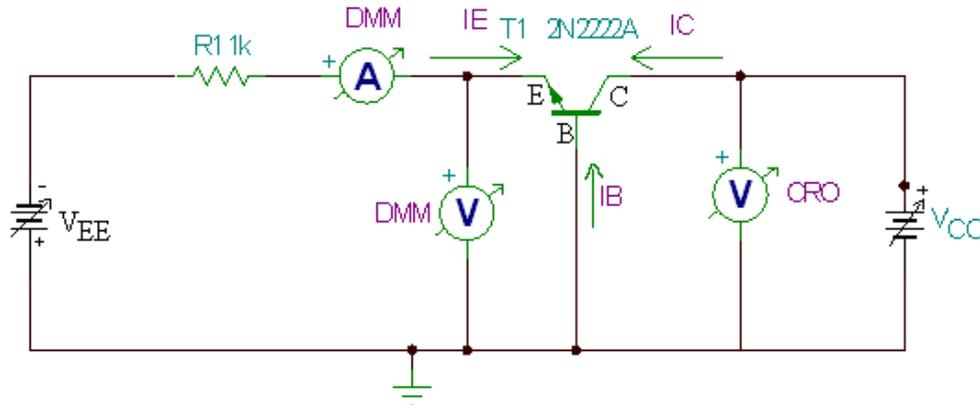
**Fig 5.1 Circuit for Common Base Input Characteristics**
