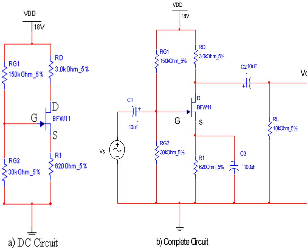
**Fig 9.1 Single Stage Common Source JFET Amplifier**
