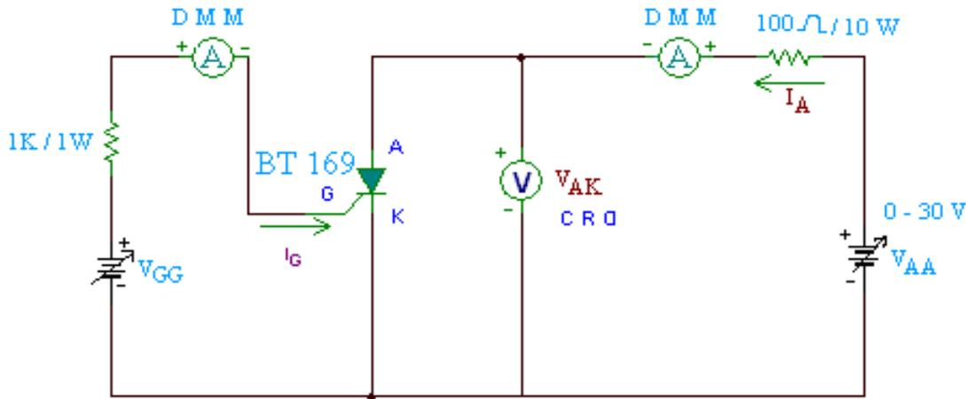
**Fig 12.1 Circuit to Plot SCR Static Characteristics.**
